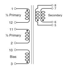
Primary windings to be connected in series and secondary windings to be connected in parallel on the PC board.
